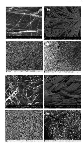
Fig. 2 SEM images of xerogels of (a)  $Zn(\shortparallel):L1$ , (b)  $Zn(\shortparallel):L2$ , (e)  $Cd(\shortparallel):L1$  and (f)  $Cd(\shortparallel):L2$ ; TEM images of xerogels of (c)  $Zn(\shortparallel):L1$ , (d)  $Zn(\shortparallel):L2$ , (g)  $Cd(\shortparallel):L1$  and (h)  $Cd(\shortparallel):L2$ .
