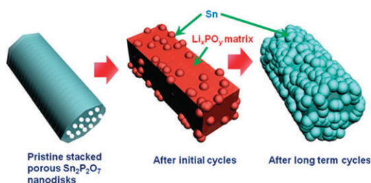
Fig. 4 Schematic view of morphology evolution of pristine stacked porous nanodisks.
