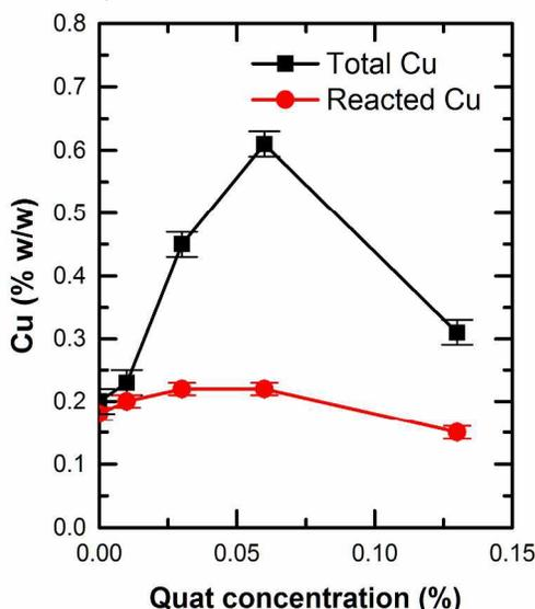
**Figure 7** Total Cu and reacted Cu concentrations of southern pine sawdust treated by 0.05% (w/w on Cu basis) MC with varying quat concentrations.
