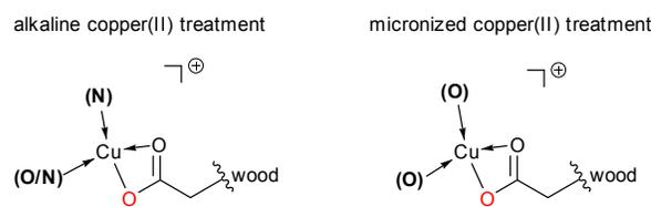
**Scheme 2** Representative model structures of fixed Cu(II) as derived from EPR studies. The resulting fixed Cu(II) species differ for alkaline copper(II) treated wood (left, EPR  $g_{||} = 2.27$ ,  $A_{||} \sim 180G$ ) and micronized copper(II) treated wood (right, EPR  $g_{||} = 2.36$ ,  $A_{||} \sim 130G$ ). The differences in EPR parameters reflect a change in the exogenous ligands (N vs. O-based) in the fixed Cu(II) complexes.
