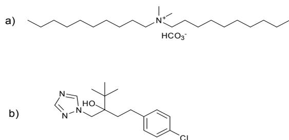
**Figure 1** Co-biocides: a) didecyldimethylammonium bicarbonate/carbonate (DDA bicarbonate/ carbonate) used in ACQ-B and ACQ-D; b) tebuconazole used in CA-B
