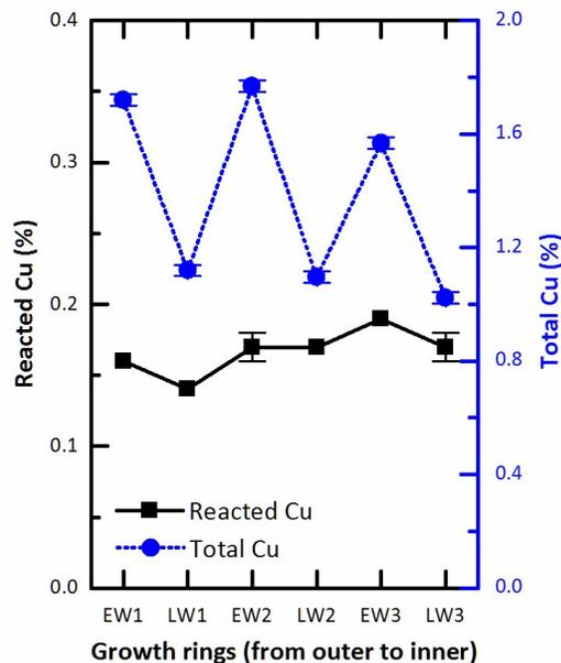
**Figure 9** Earlywood (EW) and latewood (LW) retentions of reacted Cu(II) and total Cu, measured in three consecutive rings of MCA treated red pine.
