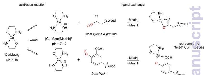
**Scheme 1** Chemical fixation of Cu(II) complexes in alkaline methanolamine treatments.
