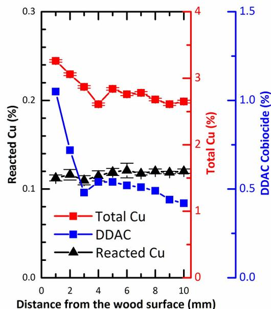
**Figure 8** Depth profiling of commercially MCQ-treated red pine. Reacted Cu, total Cu and quat content at sampling locations 0-10 mm from the wood surface.<sup>39</sup>
