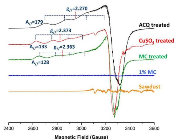
**Figure 4** EPR spectra of de-ionized water treated southern pine sawdust, micronized copper suspension containing 1% Cu, and commercial red pine sapwood treated with MC,  $CuSO_4$  and ACQ
