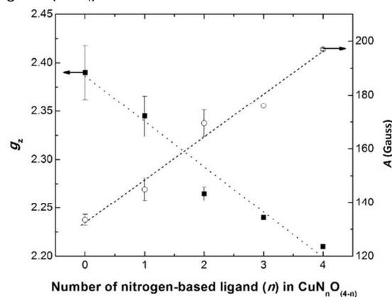
**Figure 3** The relationship between the EPR spectral parameters  $g_z$  (■) and  $A_z$  (○) for a series of Cu(II) compounds (based on data reported in Peisach and Blumberg 1974; Ruddick 1992; Ruddick et al. 2001)
