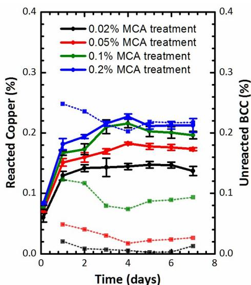
**Figure 6** Time evolution of copper(II) speciation in sawdust samples using different MCA treatment concentrations. Solid lines show profile for reacted wood concentrations (measured by EPR) whereas dashed lines show remaining unreacted BCC. Note that even at very high treatment concentrations, the total reacted copper never exceeds
