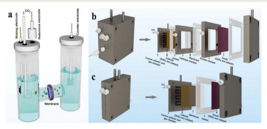
Fig. 2 Diagram of different types of eCO₂RR electrolytic cells. (a) H-type cell (b) flow cell (c) MEA. (a–c) are reproduced from ref. 59 with permission from Springer Nature Link, copyright 2023.
