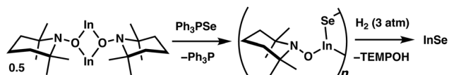
Fig. 4 Generation of a proposed oligomeric intermediate following selenium transfer from \text{Ph}_3\text{PSe} to 5 followed by the removal of the TEMPO ligands via the addition of \text{H}_2 .
