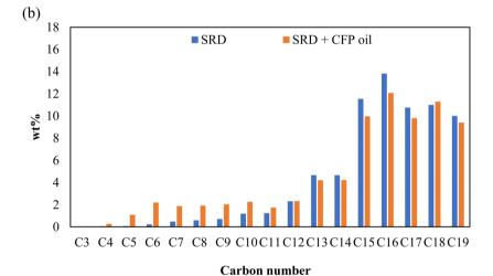
Fig. 4 (a) GC-VUV analysis of oil products from hydrotreating at 325 °C, 55 bar over sulfided NiMo/sulfided CoMo; (b) carbon number distribution of oil products from SRD hydrotreating and co-hydrotreating of SRD and CFP oil over sulfided NiMo.
