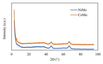
Fig. 3 XRD results of hydrotreating catalysts.
