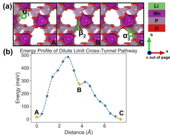
Fig. 7 Li-ion evolution of the along-tunnel pathway (PathwayII) in the dilute limit. (a) Shows images along the pathway, and Li positions labeled  $\alpha_1$ ,  $\beta_2$  and  $\alpha_3$  have the same positions with identical labels in Fig. 4. (b) Shows calculated energy evolution as a function of Li migration distance, where labels  $\alpha_1$ ,  $\beta_2$  and  $\alpha_3$  correspond to the images in (a).
