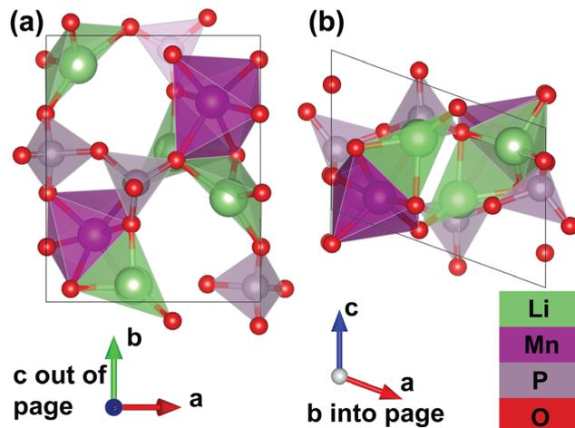
Fig. 3 The unit cell structure of the fully discharged  $\gamma$ - $\text{Li}_2\text{MnP}_2\text{O}_7$ . (a) Shows the  $c$ -axis, the tunnel direction, pointing into and out of page, and (b) shows the  $c$ -axis pointing up and down. This structure is in the  $P2_1$  spacegroup ( $a = 7.27 \text{ \AA}$ ,  $b = 8.55 \text{ \AA}$ ,  $c = 5.12 \text{ \AA}$ , and  $\alpha = 90^\circ$ ,  $\beta = 110^\circ$ ,  $\gamma = 90^\circ$ ). Identifier from the materials project: mp-770967.
