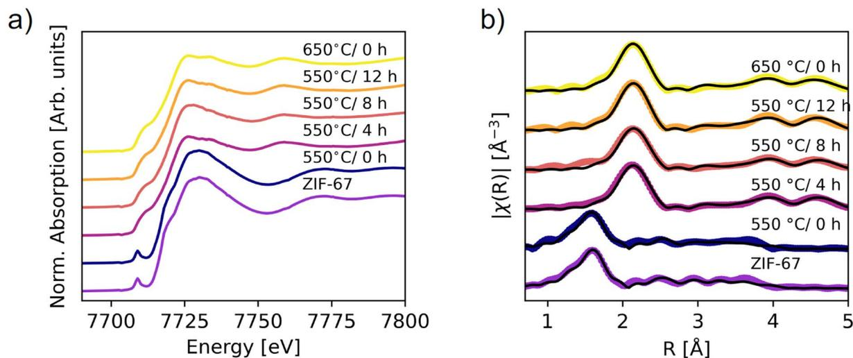
Fig. 5 XAS on the *ex situ* pyrolyzed samples. (a) XANES data. (b) Fourier transform of the EXAFS (not phase corrected). Spectra of the pristine and 550 °C/0 h samples are fitted by using scattering paths calculated from the ZIF-67 structure, while the remaining spectra are fitted with the paths from metallic Co (fcc). The scattering paths were calculated in Artemis.<sup>48</sup>
