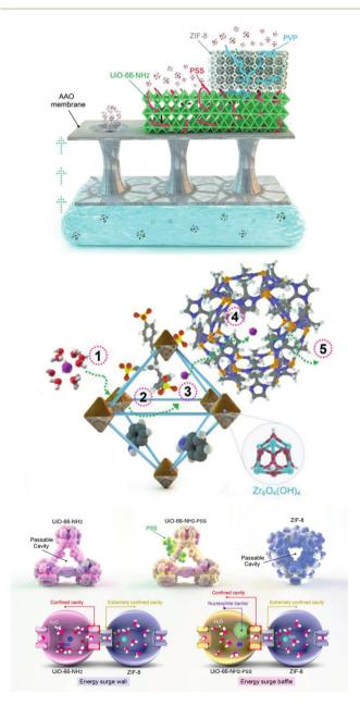
Fig. 7 Conceptual design of the asymmetrical architecture for the combination of UiO-66-NH<sub>2</sub> and ZIF-8.<sup>74</sup> Copyright 2022 Wiley-VCH.
