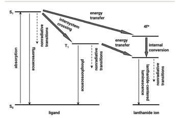
Fig. 12 Simplified energy transformation processes for the luminescent mechanism in Ln-MOFs.<sup>88</sup> Copyright 2011 American Chemical Society.
