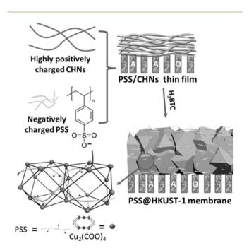
Fig. 3 Preparation of PSS@HKUST-1 membranes.<sup>67</sup> Copyright 2016 Wiley-VCH.
