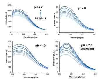
Fig. 13 Luminescent emission spectra of LMOF-321 after incremental additions of a lithium-ion aqueous solution under different pH values. 69 Copyright 2019 American Chemical Society.
