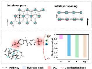
Fig. 4 Design of the PSS modified Zr-MOF for lithium-ion sieving.<sup>68</sup> Copyright 2024 American Chemical Society
