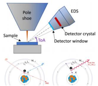
Fig. 10 Schematic system of the SEM-EDS equipment and the process of the emission of characteristic X-rays.<sup>83</sup> Copyright 2020 Elsevier.
