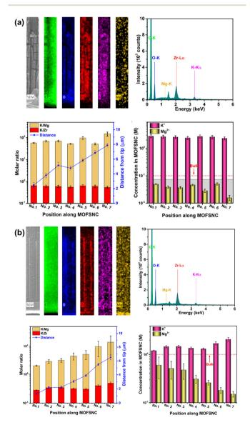
Fig. 11 SEM-EDX analysis of MOFs with (a) 0.1 M KCl + 0.1 M MqCl<sub>2</sub> and (b) 1.0 M KCl + 1.0 M MgCl<sub>2</sub> mixture solution.<sup>72</sup> Copyright 2020 Springer Nature.
