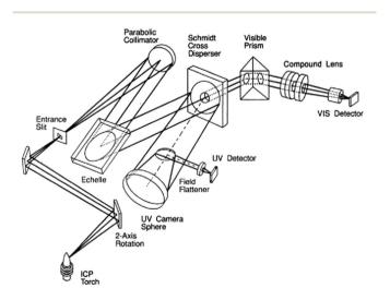
Fig. 9 Schematic optical system of the ICP-OES equipment.<sup>79</sup> Copyright 1993 American Chemical Society.
