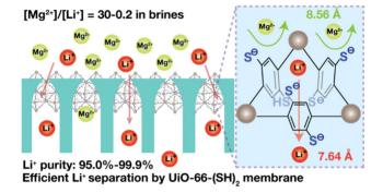
Fig. 5 Selective binding of Li<sup>+</sup> ions towards Mg<sup>2+</sup> ions by UiO-66-(SH)<sub>2</sub>.<sup>70</sup> Copyright 2024 American Chemical Society.
