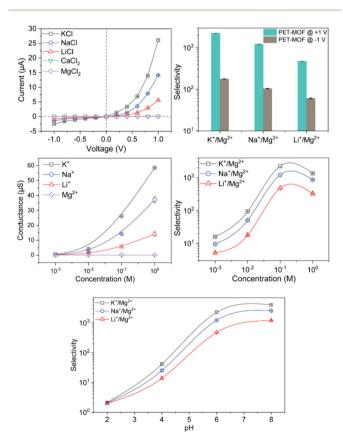
Fig. 15 Ion transport, conductance, and selectivity performance of UiO-66-(SH)<sub>2</sub> calculated by I-V measurement.<sup>70</sup> Copyright 2024 American Chemical Society.
