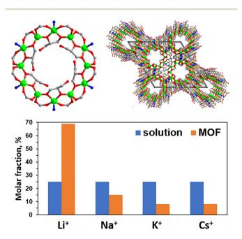
Fig. 6 Structure of the Zn<sub>12</sub>-cluster-based MOF with its selective adsorption capacities. 71 Copyright 2019 American Chemical Society.
