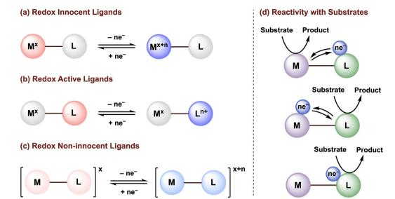
Fig. 1 Classification of (a) redox innocent, (b) redox-active, and (c) redox non-innocent ligands. (d) Possible metal-ligand cooperativity for substrate activation.
