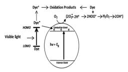
Fig. 15 Direct dye degradation.
