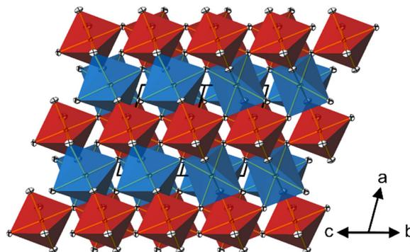
Fig. 4 Projection of the dirutile-type crystal structure of  $\text{CoTeO}_4$  along  $[011]$ .  $[\text{CoO}_6]$  octahedra are given in blue,  $[\text{TeO}_6]$  octahedra in red. Displacement ellipsoids are drawn at the 90% probability level.
