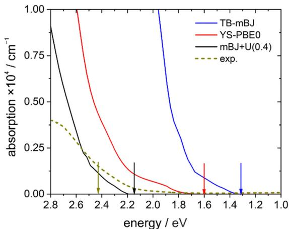
Fig. 13 Onset of the unpolarized theoretical absorption spectrum (TB-mBJ, YS-PBE0, TB-mBJ+ $U$  (4.08) functionals) in comparison with the experimental (exp.) data. The arrows mark the corresponding band gaps.
