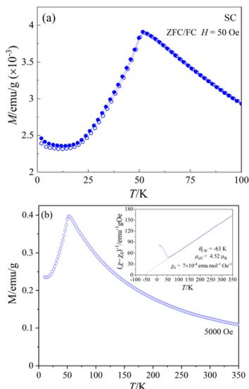
Fig. 9 (a) ZFC/FC  $M$  vs.  $T$  curves of  $\text{CoTeO}_4$  for  $H = 50$  Oe; (b)  $M(T)$  under  $H = 5$  kOe. Inset in (b) shows  $(\chi - \chi_0)^{-1}$  vs.  $T$  and linear Curie–Weiss fit in the range  $70 \leq T \leq 300$  K. The obtained parameters are indicated in the Figure.
