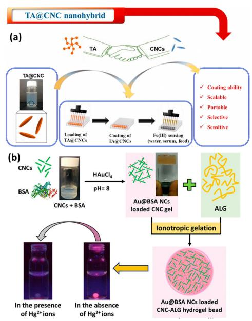
Fig. 5 Use of CNCs in metal sensing: (a) tannic acid loaded CNCs for Fe<sup>3+</sup> detection<sup>161</sup> and (b) bovine serum albumin-protected-gold-nanocluster (Au@BSA NC) loaded CNCs-alginate hydrogel beads. 162 Reproduced from ref. 161 with permission from Elsevier, copyright 2021. Reproduced from ref. 162 with permission from ACS, copyright 2016.
