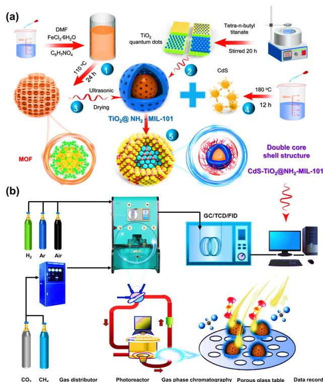
**Scheme 1** (a) Schematic diagram of the process for preparing the ternary composites; (b) process flow equipment diagram for photocatalytic  $\text{CH}_4$  dry reforming.
