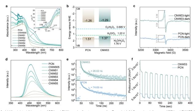
Fig. 4 (a) Ultraviolet-visible spectra of PCN and CNW samples (inset: corresponding Tauc plots). (b) Energy band diagrams of PCN and CNW03. (c) EPR signals of PCN and CNW03 under dark and light conditions. (d) Photoluminescence spectra of PCN and CNW samples. (e) Time-resolved photoluminescence spectra of PCN and CNW03. (f) Photocurrent responses of PCN and CNW03.
