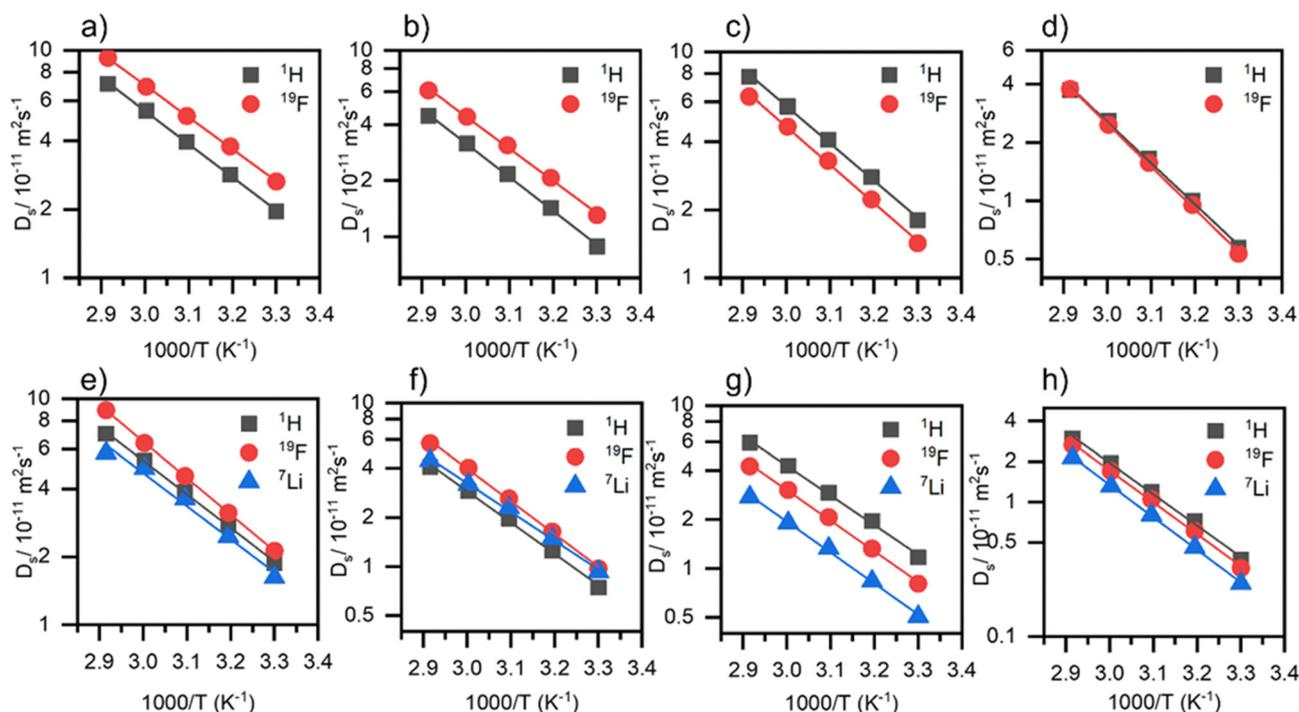
**Fig. 6** Temperature dependent self-diffusion coefficients (<sup>1</sup>H: IL cation, <sup>19</sup>F: anion, <sup>7</sup>Li: lithium cation) of neat ILs on top row in order (a) [C<sub>101</sub>mpip][FSI], (b) [C<sub>101</sub>mmor][FSI], (c) [C<sub>101</sub>mpip][TFSI], (d) [C<sub>101</sub>mmor][TFSI] and their electrolyte solutions directly below, in temperature range 30–70 °C. Errors are within the size of the data points.
