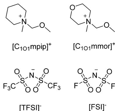
Fig. 1 Structure and abbreviations of cation and anions used. Cation abbreviations are: *N*-methoxymethyl-*N*-methylpiperidinium [C<sub>101</sub>mpip]<sup>+</sup> and 4-methoxymethyl-4-methylmorpholinium [C<sub>101</sub>mmor]<sup>+</sup>. Anion abbreviations are bis(trifluoromethanesulfonyl)imide [TFSI]<sup>-</sup>, and bis(fluorosulfonyl)imide [FSI]<sup>-</sup>.
