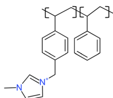
Fig. 2 Chemical structure of Sustainion membrane.
