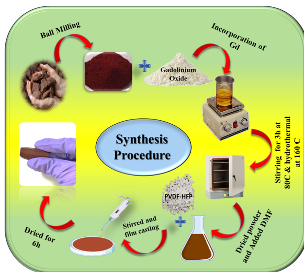
Scheme 1 Schematic representation of the synthesis procedure.
