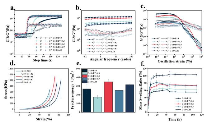
Fig. 3 Material evaluation and screening. (a) Time scan. (b) Frequency scan. (c) Strain scan. (d) Stress-strain curves for hydrogel compression tests. (e) Fracture energy of compression test. (f) Swelling test.
