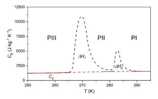
Fig. 2 Specific heat capacity,  $C_{\rm p}$ , measurements of the [DBA][BF<sub>4</sub>] material from 250 to 295 K on heating. Note: solid red lines represent the calculated  $C_{\rm p}$  for the different polymorphs in the studied temperature range; meanwhile dashed lines represent the discontinuity of  $C_{\rm p}$  across the transitions. Black dashed lines represent the transition peaks.
