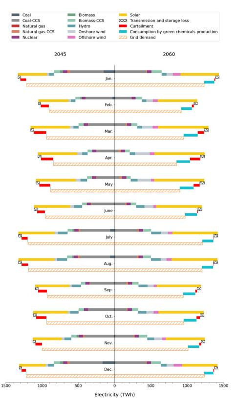
Fig. 7 Comparison of power sector monthly operation under the electricity-chemical nexus between 2045 and 2060.
