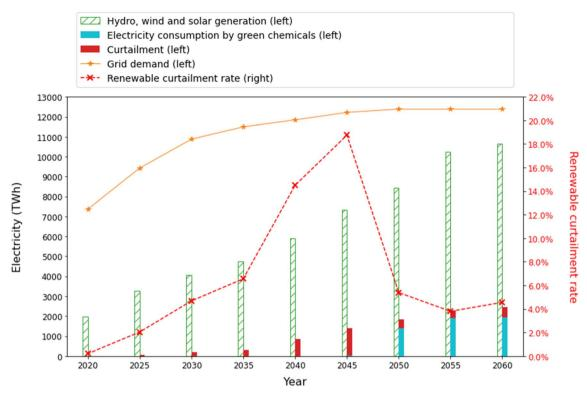
Annual renewable generation, intermediate consumption and curtailment under the electricity-chemical nexus.
