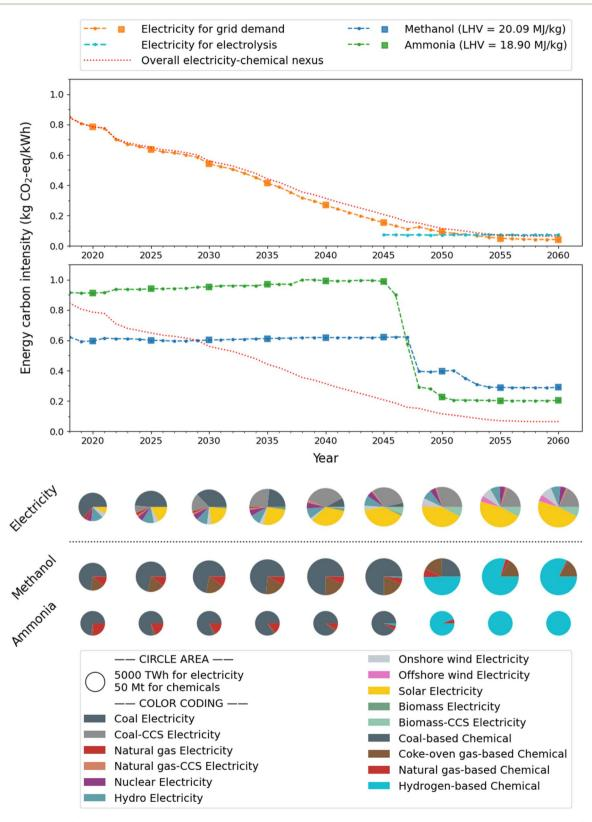
Fig. 2 Carbon intensity (top line charts with highlighting scatters for final products every 5 years) and technology mix every 5 years (bottom pie charts) along the nexus transformation pathway for electricity, methanol and ammonia.
