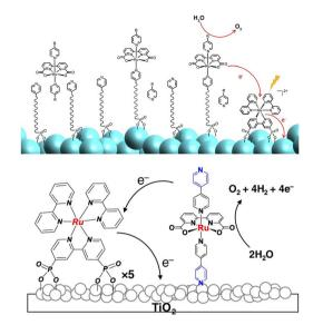
Fig. 9 Top: Coordination of a Ru(bda) WOC at MOx surfaces exploiting a long pyridine-terminated alkyl linker; the Ru trisbipyridine photosensitizer is anchored through phosphonate linkers at the bpy. Bottom: Immobilization of a Ru(bda) WOC on TiO<sub>2</sub> through a pyridine based anchoring group. Reprinted from ref. 92 with permission from the American Chemical Society, copyright 2018 and from ref. 93 with permission from the Nature Publishing Group, copyright 2020.
