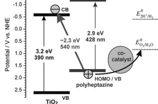
Fig. 27 (a) Hybrid photoelectrodes based on nanocrystalline  ${\rm TiO_2}$  sensitized with polyheptazine and loaded with a  ${\rm CoO_x}$  WOC, and (b) energy levels evidencing the direct optical charge-transfer excitation of an electron from the polyheptazine HOMO into the conduction band of  ${\rm TiO_2}$ . Reprinted from ref. 134 with permission from Springer, copyright 2013.
