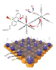
Fig. 25 Structure of the photoanode reported by Karadas and coworkers, based on the incorporation of a Prussian blue structure for the sensitization of  ${\rm TiO_2}$ , acting as an electron shuttle between a Co based catalytic centre and a phenazine-based Janus green B dye with a quaternized nitrogen. Reprinted from ref. 130 with permission from Wiley, copyright 2020.
