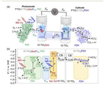
Fig. 3 (a) Representation of the photoelectrochemical cell developed by Reisner and co-workers for bias-free water oxidation and carbon dioxide reduction to formate. The photoanode is an  $IO-TiO_2|dpp|P_{Os}-PSII$  photoelectrode, while the cathode is an  $IO-TiO_2|FDH$ . (b) Energy diagram. Reprinted from ref. 65 with permission from the American Chemical Society, copyright 2018.
