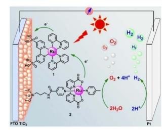
Fig. 7 Photoanode reported by Sun and co-workers, based on the ruthenium trisbipyridine dye anchored to TiO2 through phosphonate linkers and a Ru<sup>II</sup>(bda) WOC functionalized with a long insulating silatrane-terminated anchoring group. Reprinted from ref. 88 with permission from the American Chemical Society, copyright 2013.
