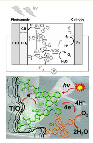
Fig. 14 Photosynthetic systems combining a Ru(bda) WOC and a subporphyrin (top) or BODIPY (bottom) photosensitizer, anchored onto a TiO2 semiconductor. Reprinted from ref. 105 and 106 with permission from the Royal Society of Chemistry, copyright 2016 and 2017.
