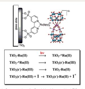
Fig. 6 Representation of a Ru trisbipyridine sensitized  $TiO_2$  photoanode with a Ru<sub>4</sub>POM catalyst assembled by electrostatic interactions, and schematic view of the photoinduced electron transfer events (1 is the Ru<sub>4</sub>POM catalyst). Reprinted from ref. 79 with permission from the Royal Society of Chemistry, copyright 2010.
