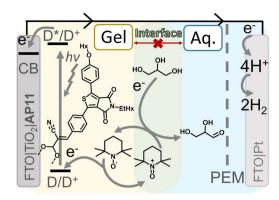
Fig. 29 Photoelectrochemical cell for glycerol oxidation and simultaneous  $H_2$  evolution proposed by Reek and co-workers. At the photoanode, the yellow and azure colours represent the redox-gel layer and the aqueous solution, respectively, while oxidation of glycerol by oxoammonium TEMPO<sup>+</sup> occurs at the interface (green area). Reprinted from ref. 156 with permission from Wiley, copyright 2022.
