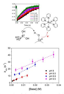
Fig. 5 Representation of photoinduced proton coupled electron transfer occurring at the surface of  ${\rm Co_3O_4}$  nanoparticles WOC, where the electron is transferred to  ${\rm Ru}^{III}({\rm bpy})_3^{-3+}$  and the proton to borate; below is reported the dependence on the rate constant on the pH and on the concentration of the borate base, indicative of a general base catalysis. Reprinted from ref. 77 with permission from the Royal Society of Chemistry, copyright 2018.
