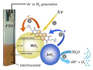
Fig. 16 A cationic perylene bisimide derivative,  $PBl^{2+}$ , absorbed on a nanostructured  $WO_3$  semiconductor and coupled to an  $IrO_x$  nanoparticle WOC, developed by Prato, Caramori and Bignozzi. Reprinted from ref. 114 with permission from the American Chemical Society, copyright 2015.
