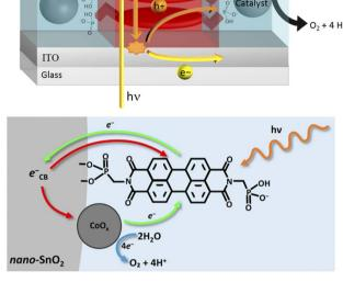
Fig. 15 Perylene bisimide (PBI) photosensitizers combined with a cobalt oxide WOC onto ITO or mesoporous  $SnO_2$ , developed by Finke and co-workers. Reprinted from ref. 111 and 112 with permission from the American Chemical Society, copyright 2017 and 2022.
