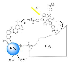
Fig. 4 Schematic representation of the photosynthetic system proposed by Mallouk and co-workers, constituted by a Ru polypyridine photosensitizer,  $IrO_x$  WOC and a benzimidazole-phenol (BIP) based redox mediator, embedded onto a  $TiO_2$  surface. Reprinted from ref. 72 with permission from the *Proceedings of the National Academy of Sciences* (PNAS), copyright 2012.
