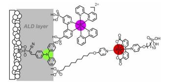
Fig. 23 Photoanodes employing a triphenylamine photosensitizer (green ball) bound to the semiconductor, a protective ALD layer used to anchor a Ru(bda) WOC (red ball) and a Ru(III) trisbipyridine redox mediator (purple ball). Reprinted from ref. 128 with permission from the *Proceedings of the National Academy of Sciences* (PNAS), copyright 2018.
