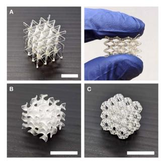
Fig. 4 Thermosets A, B, and C 3D-printed by the CLIP system. Scale  $\mbox{\rm bar}=1\mbox{ cm}.$
