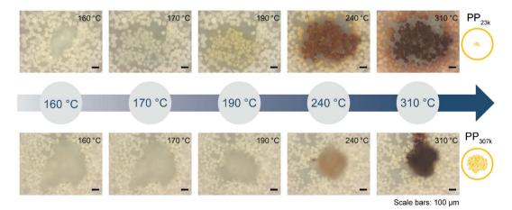
Fig. 6 In situ optical microscopy of polypropylene (PP) cracking using FCC catalyst. Individual polymer grains were placed on a bed of FCC catalyst and heated at 10 °C  $\min^{-1}$  under  $N_2$  flow in a Linkam stage. Images were acquired every minute. See ESI† for videos of the full reaction. Top: PP<sub>23k</sub>. Bottom: PP<sub>307k</sub>
