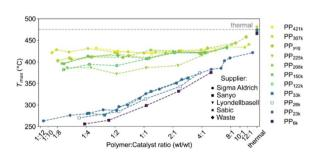
Fig. 5  $T_{\text{max}}$  for cracking of various PP samples obtained from different manufacturers using ECAT at various P:C ratios. For full thermogravimetric analysis (TGA) profiles we refer to Fig. S4 and S5.†
