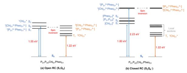
Fig. 8 Schematic representation of the singlet and triplet vertical excitation energies of the  $P_{D1}P_{D2}Chl_{D1}Pheo_{D1}$  tetramer in: (a) the open RC ( $S_1Q_A$ ), and (b) the closed RC ( $S_2Q_A$ ). All energies are reported relative to the ground state singlet ( $S_0$ ).
