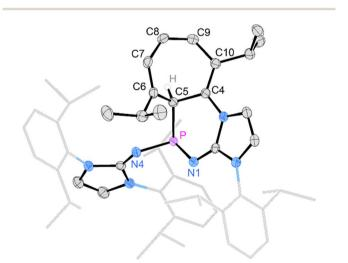
Fig. 3 Solid-state structure of **8**. Hydrogen atoms (except C5 hydrogen) are omitted for clarity. Ellipsoids are drawn at 50% probability. Dipp groups are shown in wireframe. Selected bond lengths [Å] and angles [deg]: P-C5 1.866(2), P-N1 1.7017(14), P-N4 1.693(2), C5-C6 1.510(3), C6-C7 1.358(2), C7-C8 1.433(3), C8-C9 1.366(3), C9-C10 1.438(3), C10-C4 1.366(2) C4-C5 1.510(3), N1-P-N4 199.67(7), N1-P-C5 103.78(7), C4-P-C5 100.84(7).
