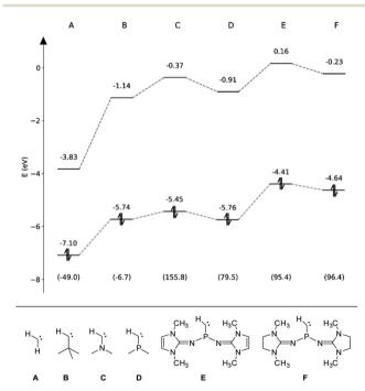
Fig. 4 Eigenenergies of the HOMO and LUMO for carbenes A–F obtained at the B3LYP-GD3BJ/def2-TZVP level. The respective singlet–triplet energy differences ( $\Delta E_{ST}$ ) are given in kJ mol<sup>-1</sup> in parentheses.
