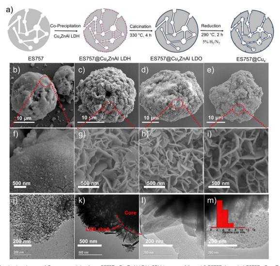
Fig. 1 (a) Synthesis scheme of Cu nanoparticles from ES757@Cu<sub>x</sub>ZnAl LDH. SEM images of (b and f) ES757; (c and q) ES757@Cu<sub>1.3</sub>ZnAl LDH; (d and h) ES757@Cu<sub>1.3</sub>ZnAl LDO and (e and i) ES757@Cu<sub>1.3</sub>. TEM images of (j) ES757; (k) ES757@Cu<sub>1.3</sub>ZnAl LDH; (l) shell of ES757@Cu<sub>1.3</sub>ZnAl LDO; (m) shell of ES757@Cu<sub>1 3</sub>.
