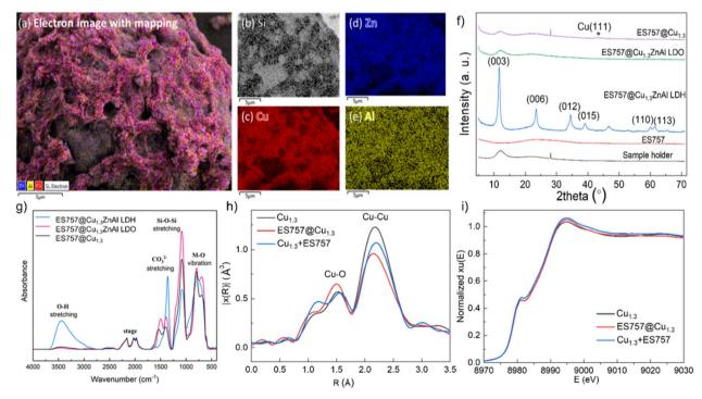
Fig. 2 Structural evolution during the preparation of ES757@Cu<sub>1.3</sub>. (a) Electron image with Zn, Al, Cu, Si element mapping; (b) Si; (c) Cu; (d) Zn; (e) Al of ES757@Cu<sub>1.3</sub>ZnAl LDH; (f) powder X-ray diffraction patterns; (g) FTIR spectra; (h) Fourier transformed magnitudes of the experimental Cu K-edge EXAFS spectra; (i) normalised Cu K-edge XANES spectra.
