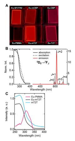
Fig. 3 Optical properties of Eu(hfa)<sub>3</sub>(TPPO)<sub>2</sub>-doped films. (A) Photos of emission from the fabricated films upon photoexcitation with 254 nm. (B) Absorption (solid line), excitation probed at 615 nm (broken line), and emission (red line) spectra of the Eu-mT2T film. (C) Absorption spectra of the Eu-PMMA film (pink line), Eu-mT2T film (black line), and mT2T neat film (sky blue line)
