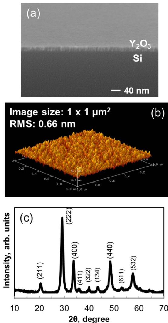
Fig. 7 (a) FE-SEM image of  $\text{Y}_2\text{O}_3$  film deposited onto Si substrate at 200 °C. (b) Three-dimensional AFM image of  $\text{Y}_2\text{O}_3$  film deposited onto Si substrate at 200 °C. (c) XRD pattern for  $\text{Y}_2\text{O}_3$  film on Si substrate. The reflections were indexed on the basis of PDF card no. 151761.
