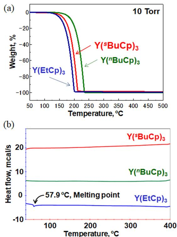
Fig. 3 (a) TGA curves for Y(<sup>5</sup>BuCp)<sub>3</sub> and conventional precursors Y(EtCp)<sub>3</sub> and Y(<sup>n</sup>BuCp)<sub>3</sub> (b) DSC thermograms of Y(<sup>5</sup>BuCp)<sub>3</sub> and conventional precursors Y(EtCp)<sub>3</sub> and Y(<sup>n</sup>BuCp)<sub>3</sub>.
