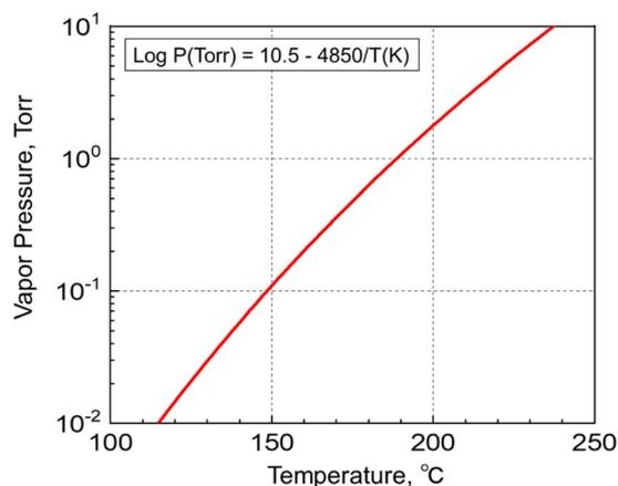
Fig. 2 Vapor pressure variations of Y(<sup>5</sup>BuCp)<sub>3</sub> with temperature.
