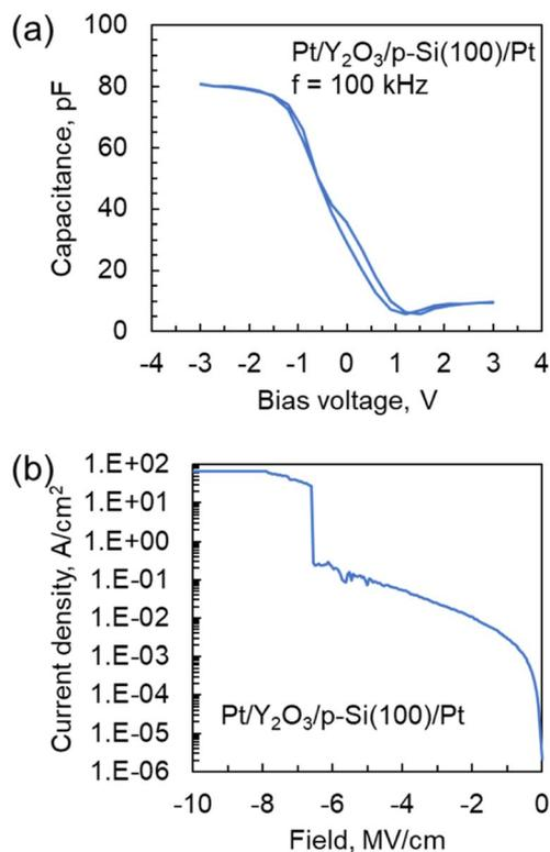
Fig. 8 (a)  $C$ – $V$  and (b) leakage current density vs. electric field curves for the Pt/ $\text{Y}_2\text{O}_3$ /p-Si capacitor. The deposition temperature for the  $\text{Y}_2\text{O}_3$  layer was 300 °C.
