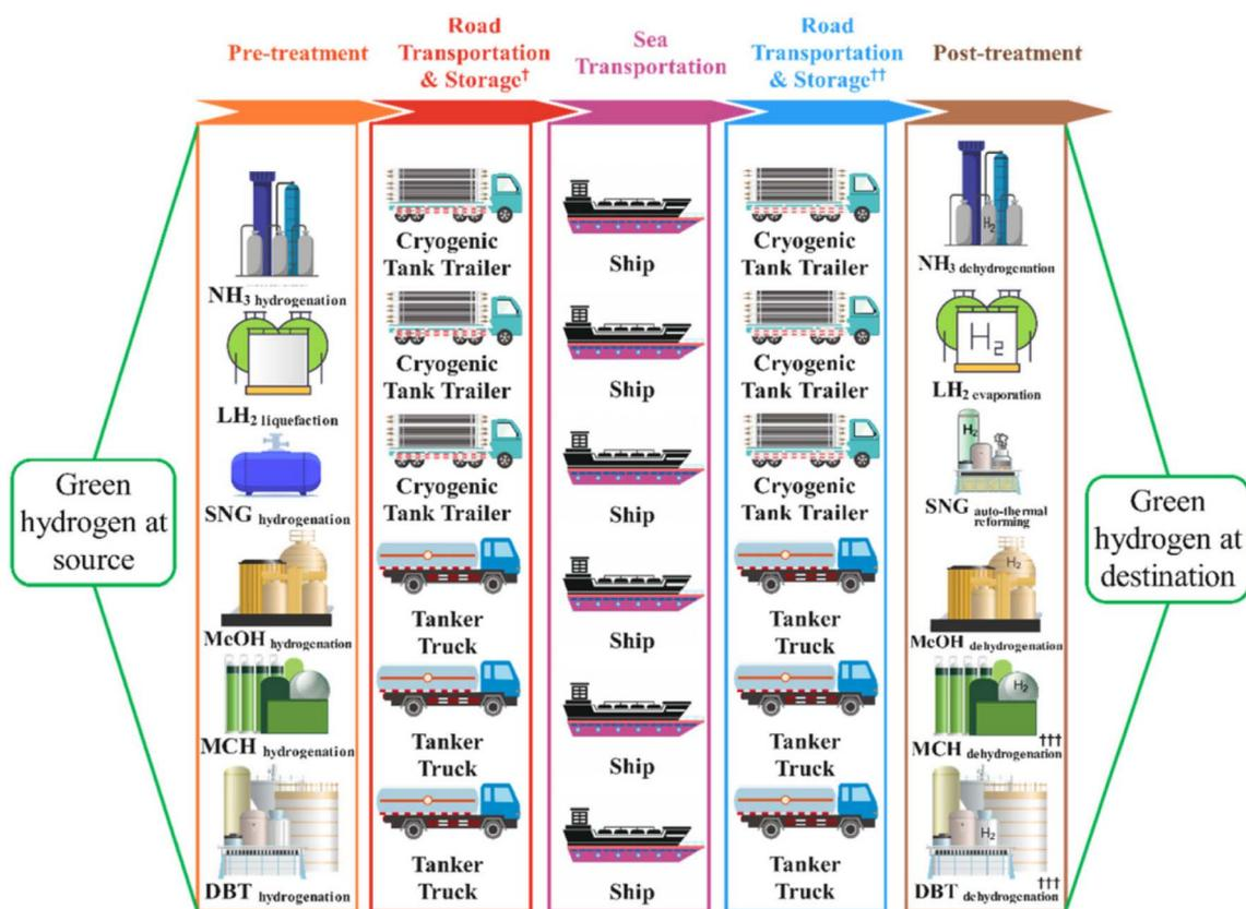
Fig. 21 A schematic of the hydrogen delivery pathways.<sup>135</sup> Reproduced from ref. 135 with permission from [Royal Society of Chemistry], copyright [2022].
