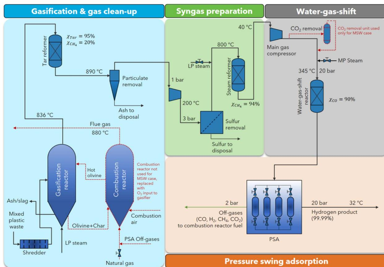
Fig. 12 Schematic of flow diagram of gasification process using mixed plastic waste precursor to produce hydrogen and other species.<sup>94</sup> Reproduced from ref. 94 with permission from [Royal Society of Chemistry], copyright [2023].
