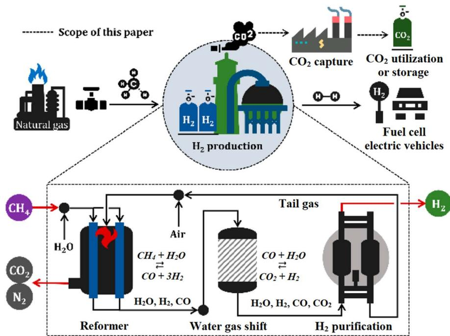
Fig. 6 Diagram of steam methane reforming for industrial hydrogen production.<sup>31</sup> Reproduced from ref. 31 with permission from [MDPI], copyright [2021].
