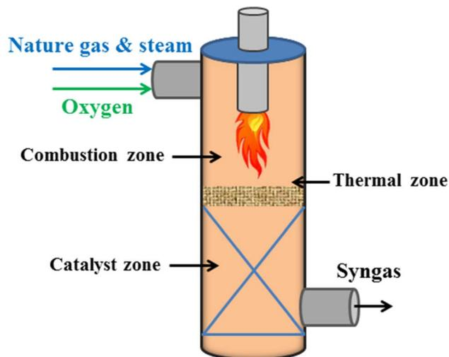
Fig. 8 Schematic of an autothermal reactor.
