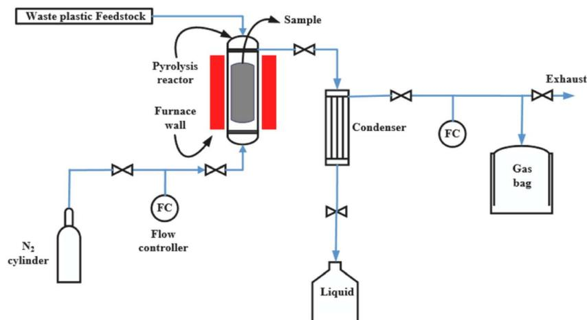
Fig. 13 A scheme of pyrolysis process to produce hydrogen from waste plastic resources.<sup>99</sup> Reproduced from ref. 99 with permission from [Elsevier], copyright [2023].
