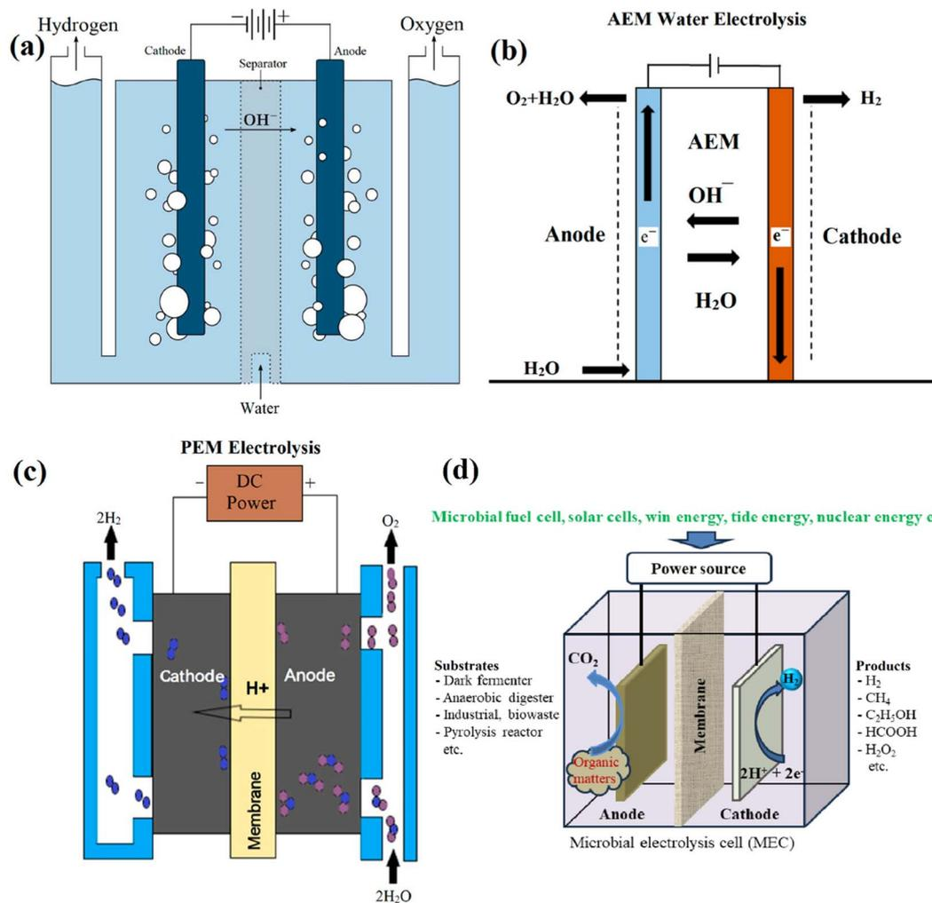
Fig. 15 Scheme of low temperature water electrolysis: (a) alkaline electrolyzers, (b) anion exchange electrolyzers, and (c) proton exchange membrane electrolyzers<sup>115</sup> Fig. 15(a)–(c) reproduced from ref. 113 with permission from [MDPI], copyright [2023] and (d) microbial electrolysis cell system.
