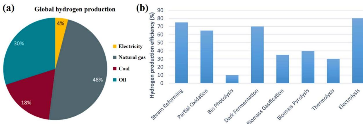
Fig. 2 (a) Global hydrogen production,<sup>16</sup> reproduced from ref. 16 with permission from [MDPI], copyright [2022] and (b) hydrogen production efficiency from various different process.<sup>17</sup> Reproduced from ref. 17 with permission from [Royal Society of Chemistry], copyright [2023].
