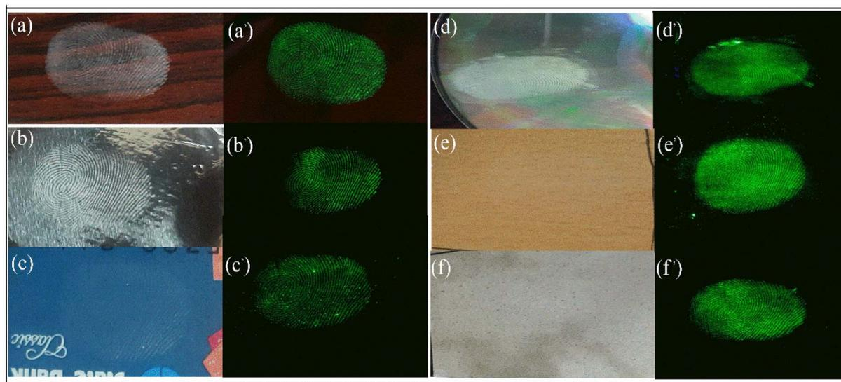
Fig. 11 Fingerprint detection using synthesized  $\text{CaYF}_5:\text{Ho}^{3+}/\text{Yb}^{3+}$  upconversion phosphor on various surfaces before (left) and after 980 nm illumination (right) (a, a') on a glass slide, (b, b') on aluminum foil, (c, c') on a debit card, (d, d') on compact disk (CD), (e, e') on a wooden block, (f, f') on ceramic tile.
