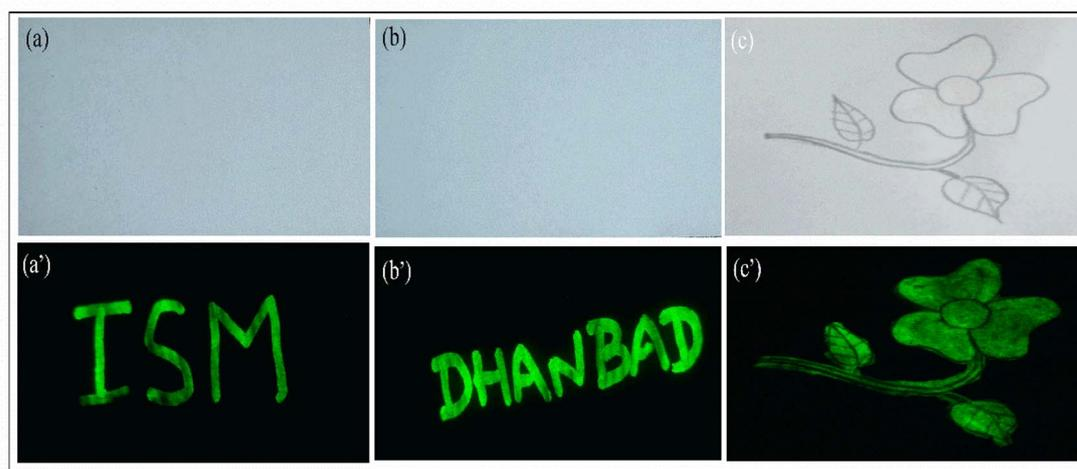
Fig. 12 Demonstration of security ink for anti-counterfeiting applications using synthesized  $\text{CaYF}_5:\text{Ho}^{3+}/\text{Yb}^{3+}$  upconversion phosphor. (a), (b), and (c) is before NIR illumination while (a'), (b'), and (c') is after NIR illumination.
