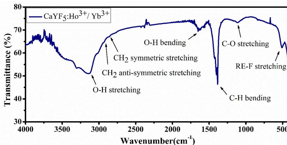
Fig. 4 FTIR spectrum of synthesized  $\text{CaYF}_5:\text{Ho}^{3+}/\text{Yb}^{3+}$  sample.
