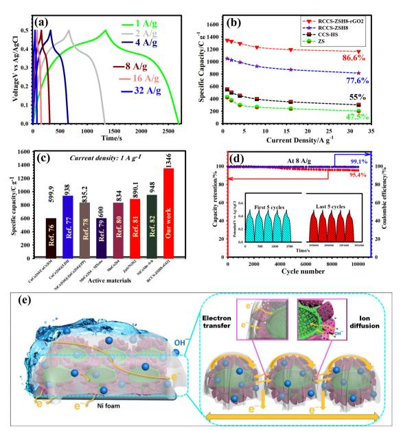
Fig. 7 (a) GCD profiles of the RCCS-ZSH8-rGO2 electrode from 1 to 32 A q<sup>-1</sup>. (b) Specific capacities vs. current densities of the ZS, CCS-HS, RCCS-ZSH8, and RCCS-ZSH8-rGO2 electrodes. (c) Comparison of capacity values of RCCS-ZSH8-rGO2 with the previous literature. (d) Longevity and Coulombic efficiency of the RCCS-ZSH8-rGO2 at 8 A g<sup>-1</sup> (the inset depicts the first and last 5 GCD cycles). (e) Schematic representation of the working mechanism of RCCS-ZSH8-rGO2 base-electrode.
