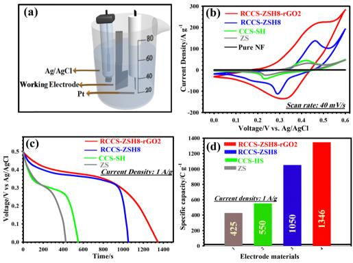
Fig. 5 (a) Schematic illustration of the three-electrode cell. (b) CV curves of the pure nickel foam, ZS, CCS-HS, RCCS-ZSH8, and RCCS-ZSH8-rGO2 electrodes at 40 mV s $^{-1}$ . (c) Discharge curves of the ZS, CCS-HS, RCCS-ZSH8, and RCCS-ZSH8-rGO2 electrodes at 1 A g $^{-1}$ . (d) Specific capacities of ZS, CCS-HS, RCCS-ZSH8, and RCCS-ZSH8-rGO2 electrodes at 1 A g<sup>-1</sup>.
