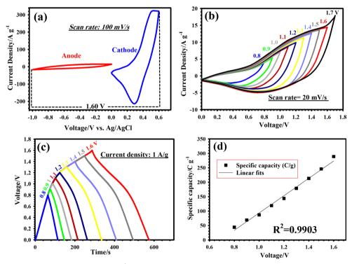
Fig. 9 (a) CVs of AC and RCCS-ZSH8-rGO2 at 100 mV s<sup>-1</sup> in a three-electrode cell. (b) CV and (c) GCD plots of RCCS-ZSH8-rGO2//AC measured in several voltage windows at a scan rate of 20 mV  $s^{-1}$  and a current density of 1 A  $g^{-1}$ , respectively. (d) Estimated specific capacity plots based on the voltage windows for RCCS-ZSH8-rGO2//AC at 1 A  $g^{-1}$ .
