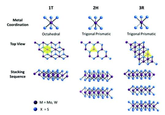
Fig. 3 Different structures and stacking orders of MoS<sub>2</sub> adapted from ref. 3 and 15 with permission from Elsevier, copyright 2021.
