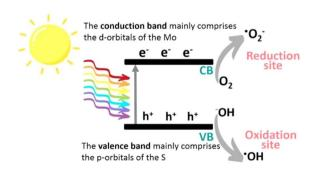
Fig. 8 Schematic illustration of the photocatalytic mechanism of MoS<sub>2</sub>.<sup>94</sup> Adapted with permission from (*ACS Omega*, 2022, 7(26), 22089–22110). Copyright (2022) American Chemical Society.
