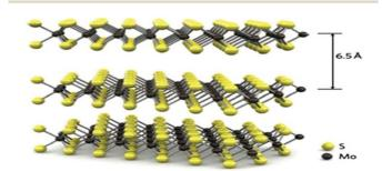
Fig. 2 Crystalline structure of MoS<sub>2</sub>, adapted from ref. 2 from Springer Nature, copyright 2014 (Owned by Springer Nature).
