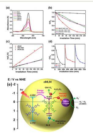
Fig. 7 (a) Absorption spectra of Rh B solution in the presence of  $\rm H_2O_2$  and nMLM; (b) visible-light photocatalytic degradation curve of Rh B over nMLM, nPCN-222, and nNU-1000; (c) kinetic study of the degradation process over nMLM, nPCN-222, and nNU-1000; (d) recycling test for nMLM; (e) proposed mechanism for rhodamine B (Rh B) degradation using nMLM.  $^{157}$  This figure has been adapted from ref. 157 with permission from American Chemical Society, copyright 2020.
