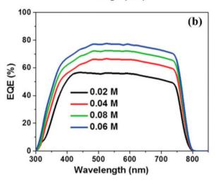
Fig. 13 (a) J-V, and (b) EQE properties of PSCs as a function of precursor concentration 0.02 M, 0.04 M, 0.08 M, 0.06 M (reproduced with permission from ref. 145. Copyright 2014 RSC).
