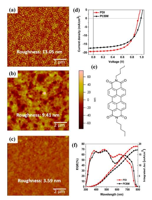
Fig. 18 AFM pictures of perovskite absorber  $(CH_3NH_3Pbl_{3-x}Br_x)$  (a) prepared on PEDOT:PSS film, (b) after fabrication of PCBM, and (c) PDI film on PEDOT:PSS/perovskite thin layer. (d) J-V curves, (e) PDI molecular assembly, and (f) EQE-wavelength findings for both PCBM and PDI ETL-based PSCs (reproduced with permission from ref. 164. Copyright 2017 Elsevier).
