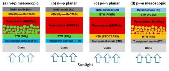
Fig. 4 Diagram displaying the four-layered assemblies of PSCs (a) n-i-p mesoscopic, (b) n-i-p planar, (c) p-i-n planar, and (d) p-i-n mesoscopic ostructured (reproduced with permission from ref. 36, copyright 2016 SPIE).
