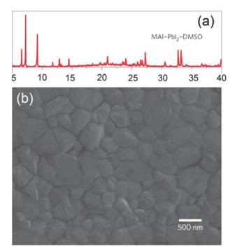
Fig. 26 (a) X-ray diffraction shape of an MAI-PbI<sub>2</sub>-DMSO intermediate stage produced by toluene treatment on the layer deposited by spin-coating of MAI-PbI<sub>2</sub>-DMSO-GBL solution. (b) SEM image of the subsequent perovskite layer using the middle stage (reproduced with permission from ref. 209 Copyright 2014 NPG).
