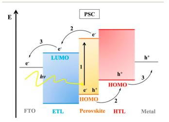
Fig. 3 Band plan and working mechanism of PSCs (reproduced with permission from ref. 32, copyright 2017 Elsevier).
