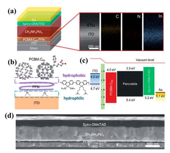
Fig. 16 (a) Illustrative depiction of the produced thin-film assembly and SEM image with EDS plotting of the cross-section of ITO/PCBM: $C_{60}$ :PFN (approx 120 nm). (b) Symbolic drawing of vertical phase parting in the ternary PCBM: $C_{60}$ :PFN and molecular structure of PFN. (c) Energy figure, and (d) SEM image showing the side view of the established device (reproduced with permission from ref. 159. Copyright 2018 RSC).
