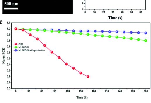
Fig. 32 (a) Side view SEM image of the PSC fabricated using MLG/ZnO. (b) PCE curve with time under maximum power point tracking. (c) Stability test of PSCs based on ZnO, MLG/ZnO, and MLG/ZnO with passivation under constant illumination for 300 hours at room temperature and under nitrogen flow (reproduced with permission from ref. 235. Copyright 2019 RSC).
