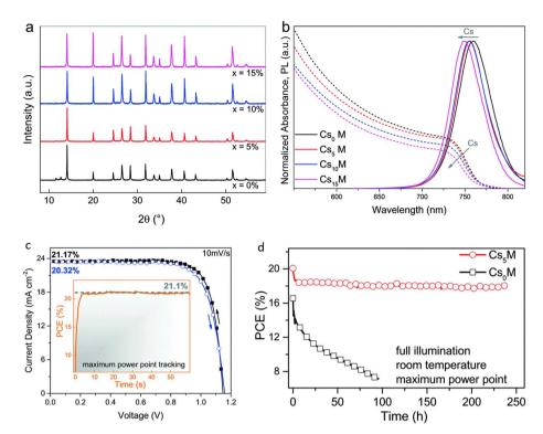
Fig. 8 Consequences of Cs accumulation in MA/FA cation blends; (a) XRD and (b) optical findings (c) current-voltage (J-V) and (d) stability properties of Cs<sub>x</sub>MAFA complexes (reproduced with permission from ref. 60. Copyright 2017 RSC)
