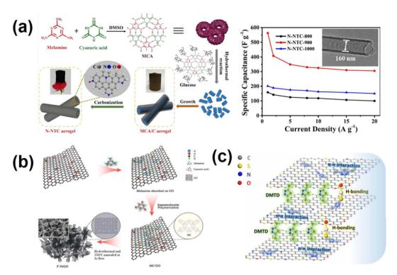
Fig. 2 (a) Schematic illustration of the synthesis and rate performance of the N-NTC aerogel.<sup>60</sup> Copyright 2021, American Chemical Society. (b) Schematic illustration of the supramolecular polymerization method for preparing P-NrGO materials.<sup>88</sup> Copyright 2018, Elsevier. (c) Schematic illustration of the interactions between GO and DMTD molecules.<sup>91</sup> Copyright 2020, Elsevier.
