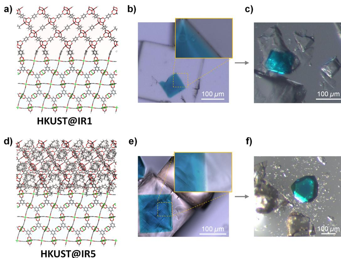
Fig. 1 Computational structural models for (a) HKUST@IR1 and (d) HKUST@IR5 MOF-on-MOFs. Green: Cu; black: Zn; grey: C; white: H; red: O. Optical microscopy images for (b and c) HKUST@IR1 and (e and f) HKUST@IR5. Images showing the interface (b and e) before and (c and f) after the crush experiment. The insets represent the seamless interface.
