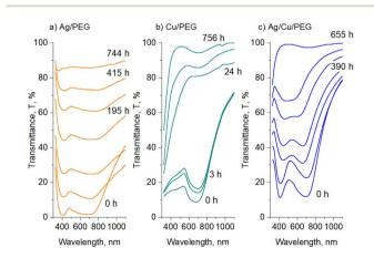
Fig. 5 Time evolution of the UV-vis transmittance spectra of: (a) Ag/ PEG, (b) Cu/PEG, and (c) Ag/Cu/PEG nanofluids. The NP mean size is 30 nm, the total metal concentration is 50  $\mu$ g mL<sup>-1</sup> (25  $\mu$ g mL<sup>-1</sup> Ag and 25  $\mu$ g mL<sup>-1</sup> Cu, in the case of Ag/Cu/PEG).
