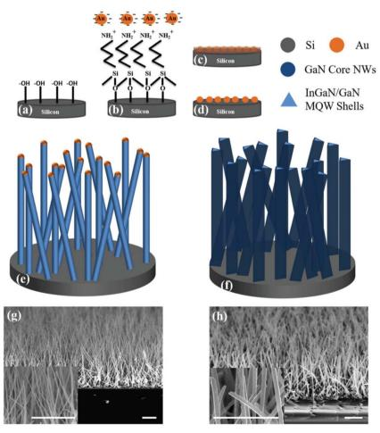
Fig. 2 Schematic depiction of catalyst preparation: (a) hydroxylation, (b) silanization and Au NP deposition, (c) in situ Ga and In deposition, and (d) annealing. The schematic for (e) VLS development of GaN core nanowires and (f) lateral growth of GaN/InGaN MQW shells around the GaN core nanowires. SEM images of (q) GaN core NWs and (h) GaN/InGaN MQW coaxial NWs, with insets showing high-magnification images in each case. Reproduced with permission from ref. 79. Copyright 2019 RSC publisher.
