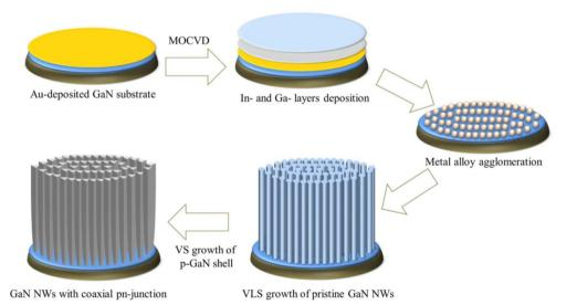
Fig. 12 Growth schematics of pristine and coaxial GaN NWs on a GaN thin film. Reproduced with permission from ref. 87. Copyright 2021 Elsevier publisher.
