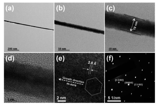
Fig. 6 Transmission electron micrographs of GaN core NWs grown on a BeO substrate: (a-c) low- to high-magnification images, (d) highmagnification image showing planes with the complete width, (e) interplanar spacing along the m-axis with a very clear growth direction, and (f) SAED patterns verifying the growth direction along the m-axis. Reproduced with permission from ref. 81. Copyright 2020 ACS publisher.
