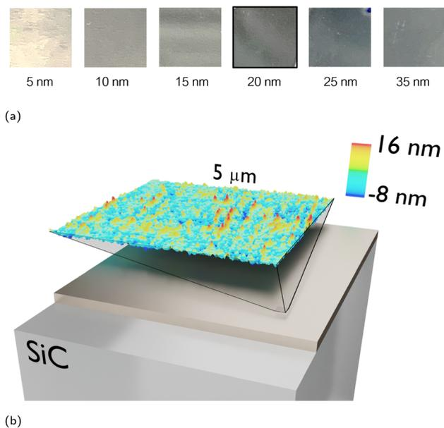
**Fig. 5** Fabricated samples. (a) Photos of the samples with increasing Ti film thickness, deposited on top of a  $220\ \mu\text{m}$  SiC wafer. (b) Detail of a  $25\ \mu\text{m}^2$  roughness of the selected sample (20 nm Ti thin film) measured *via* AFM. The RMS roughness is 2.188 nm, mean roughness is 1.635 nm, maximum peak height is 16.05 nm, maximum pit depth is 7.73 nm and the maximum height is 23.78 nm.
