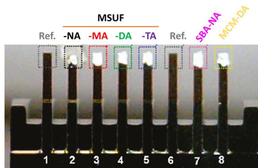
Fig. 8 Optical microscopy image of the sorbent-coated microcantilever array. Reprinted (adapted) with permission from reference *Environ. Sci. Technol.*, 2011, 45(13), 5704–5709.<sup>192</sup> Copyright 2011 American Chemical Society.
