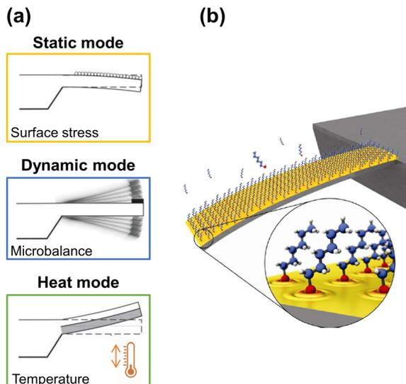
**Fig. 1** (a) Working modes of cantilever-based sensors. Adapted from ref. 32 (under a Creative Commons license CC BY-NC-ND 3.0); (b) artistic view of an alkanethiol self-assembled monolayer (SAM) on a gold-coated microcantilever formed from the gas phase. Reprinted with permission from reference *Nanotechnology*, 2010, **21**, 075501.<sup>33</sup> Copyright 2010 IOP Publishing.
