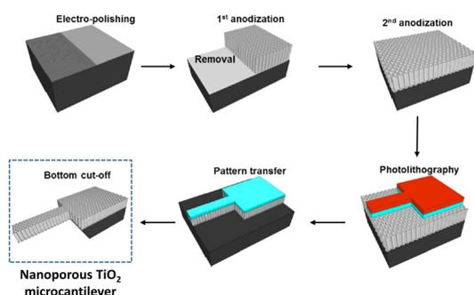
Fig. 6 Schematic illustration of the fabrication process of a nanoporous TiO<sub>2</sub> microcantilever. Reprinted (adapted) with permission from *Anal. Chem.*, 2014, **86**(10), 5077–5082.<sup>165</sup> Copyright 2014 American Chemical Society.
