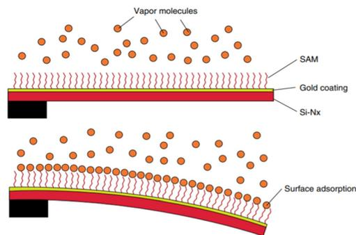
Fig. 5 Schematic diagram of a cantilever bending due to differential adsorption of analyte molecules. Reprinted with permission from reference Elsevier, 2007, pp. 109–130.<sup>156</sup> Copyright 2007 Elsevier.
