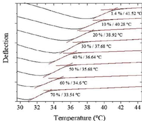
**Fig. 3**  $T_g$  variation (from 42 °C to 34 °C) as a function of humidity in the range between 1.4% and 70%. Reprinted with permission from reference *Polym. Test.*, 2018, **65**, 407–413.<sup>112</sup> Copyright 2018 Elsevier.
