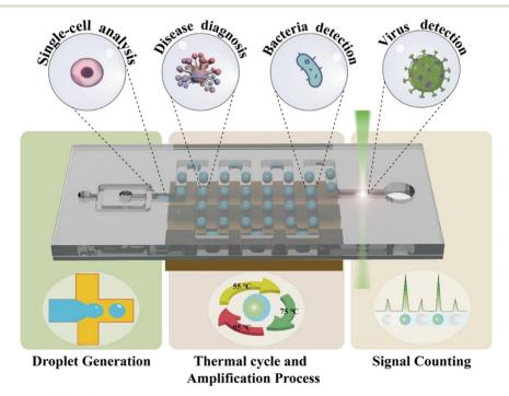
Fig. 1 Schematic diagram of ddPCR and applications.
