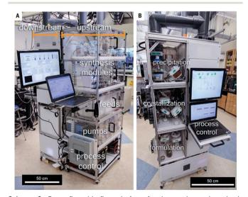
Scheme 6 Reconfigurable flow platform for the on-demand synthesis of some APIs from Jamison, Jensen and Myerson: A. Details of the upstream section of the flow platform featuring feeds, pumps, synthesis modules, and process controls. B. Details of the downstream section of the flow platform featuring precipitation, crystallization, and formulation modules.<sup>73</sup> Copyright 2016 The American Association for the Advancement of Science.
