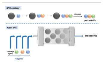
Scheme 7 Automated synthesis of prexasertib and derivatives enabled by continuous-flow solid-phase synthesis (SPS).<sup>76</sup>
