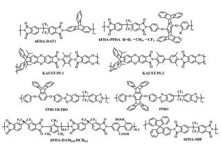
**Fig. 4** Representative chemical structures of microporous polyimides and thermally rearranged (TR) polymers.
