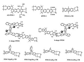
Fig. 2 Representative chemical structures of ladder-type PIMs.
