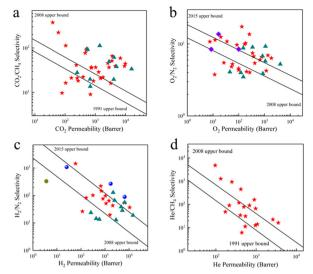
Fig. 6 Gas separation performance of CMS membranes for (a) CO<sub>2</sub>/  $CH_4,\ (b)\ O_2/N_2,\ (c)\ H_2/N_2,\ and\ (d)\ He/CH_4$  gas pairs. The red stars represent PI-based CMSMs,  $^{78,85-94}$  navy spheres represent PIM-based CMSMs, 95,96 violet diamonds represent PBI-based CMSMs, 97 dark yellow hexagon represents PFA-based CMSMs, 98 and turquoise triangles represent polypyrrolone-based CMSMs.99
