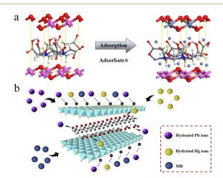
Fig. 5 (a) Schematic diagram of Ni<sup>2+</sup> adsorption with EDTAintercalated MgAl-LDH nanosorbents. Reprinted with permission from ref. 69. Copyright 2019, American Chemical Society. (b) Schematic illustration of PAAS EDTA-intercalated MgAl-LDH nanosorbents for the adsorption of Pb<sup>2+</sup> and Hg<sup>2+</sup>. Reprinted with permission from ref. 71. Copyright 2021, Elsevier.
