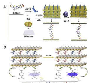
Fig. 3 (a) Schematic of fluorimetric Cd2+ detection using an ultrathin film from ZnAl-LDH nanosheets and ABTS. Reprinted with permission from ref. 54. Copyright 2011, American Chemical Society. (b) Schematic illustration of fluorescence turn-on Cr(vi) based on Fe(CN)<sub>6</sub><sup>4-</sup>-intercalated NiAl-LDHs and TA. Reprinted with permission from ref. 58. Copyright 2020, Elsevier.
