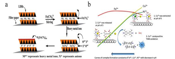
Fig. 2 (a) Illustration of the concept for the formation of  $Fe(CN)_6^{4-}$  anion-interlayered MgAl-LDH-modified test strips and the detection of heavy metal ions. Reprinted with permission from ref. 44. Copyright 2016, Elsevier. (b) Schematic of the selective extraction-release-catalysis detection process. Reprinted with permission from ref. 45. Copyright 2015, Elsevier.
