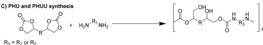
Fig. 11 Polyhydroxiuethane (PHU) and PHUU synthetic route.
