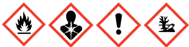
Fig. 5 Hazard pictograms for limonene in European Union countries (from left to right): GH502 (flammable); GH508 (serious health hazard); GH507 (health hazard); GH509 (hazardous to the environment).
