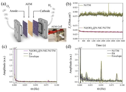
Fig. 4 (a) Schematic representation and photograph of an AEM water electrolyser. (b) Dynamic resistance variation at 10 kHz and 500 mA cm<sup>-2</sup> and the corresponding FFT plots of (c) Ni(OH)<sub>2</sub>@N-NiC/Ni/TM, and (d) Ni/TM, each used as both anode and cathode.
