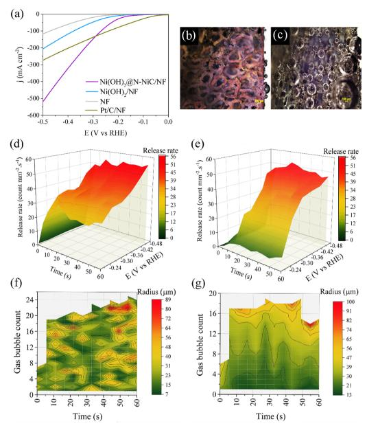
Fig. 2 (a) HER polarization curves. Optical images of gas bubbles over (b)  $Ni(OH)_2(NF)$  and (c)  $Ni(OH)_2/NF$  at 0.245 V vs. RHE. Operando optical microscopy: 3D surface plots of (d)  $Ni(OH)_2(NF)$  and (e)  $Ni(OH)_2/NF$ . Contour plots at 0.445 V vs. RHE for (f)  $Ni(OH)_2(NF)$  and (g)  $Ni(OH)_2/NF$ .
