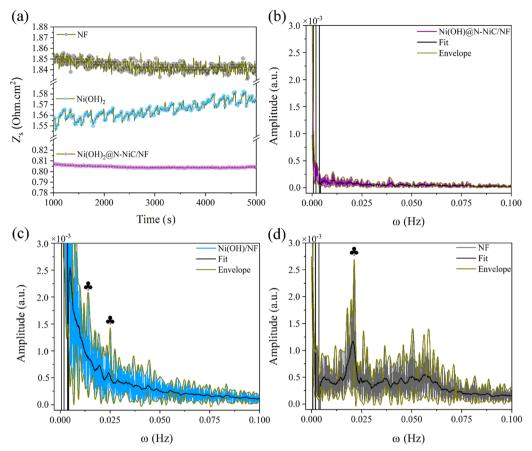
(a) Dynamic resistance variation at 20 kHz and -100 mA cm<sup>-2</sup> and the corresponding FFT plots of (b) Ni(OH)<sub>2</sub>@N-NiC/NF, (c) Ni(OH)<sub>2</sub>/NF, and Fia. 3 (d) NF.
