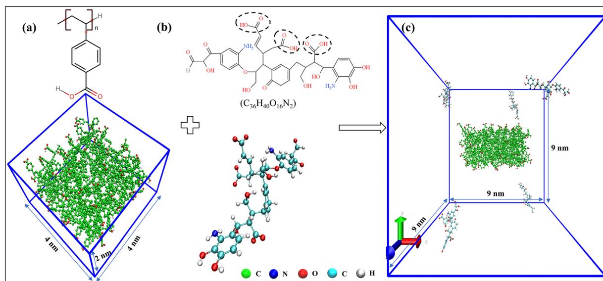
**Fig. 1** Snapshots of the simulation models (a) PS-slab; (b) TNB molecule; (c) representative unit of a simulation cell depicting the starting structure of MD simulation, water molecules are not shown here for visual clarity.
