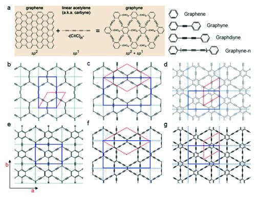
Fig. 9 Chemical structures and nomenclature. (a) Structure schematics of graphene and graphynes. (b)  $\alpha$ -graphyne; (c)  $\beta$ -graphyne; (d)  $\gamma$ -graphyne; (e) 6,6,12-graphyne; (f) β-graphdiyne; and (g) GDY.<sup>89</sup> Reused with permission from Royal Society of Chemistry.
